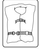
Type III, Flotation-aid Life vest is designed so that conscious wearers can turn face-up. Designed for comfort while engaged in water skiing or other forms of water activities.
