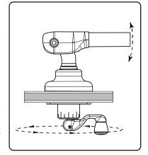
With the handle in the down position, rotate the handle clockwise to raise or lower the outrigger to the desired position.
