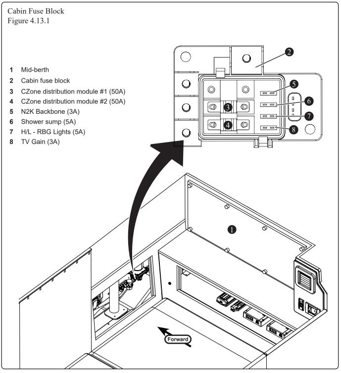
NOTE: This symbol [7A] indicates the specific amperage of the item shown (e.g., 5A = 5 amps)
