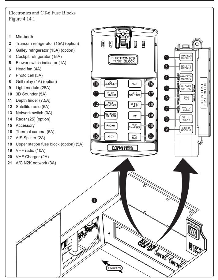
NOTE: This symbol [2A] indicates the specific amperage of the item shown (e.g., 5A = 5 amps)
