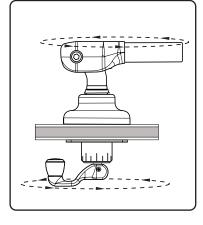
To rotate outriggers in/out: Flip the handle to the up position. Grab firmly on the handle and rotate the handle to position the outrigger to the desired position. Keep the handle in the down position to keep the base from rotating while fishing and running.
