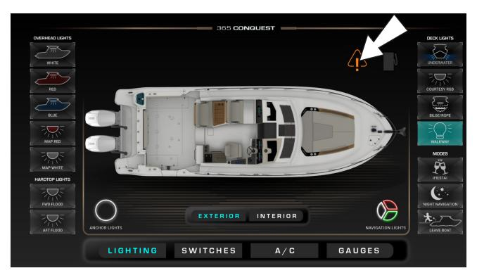
When accessing the ALARM PAGE tap DIAGNOSTIC to see component status. A green STATUS light indicates FUNCTIONS operating properly. A red STATUS light indicates FUNCTIONS requiring attention.
