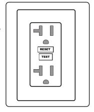
If equipped, all readily accessible 220V outlets (international only) are protected by a residual current circuit breaker (RCBO). This current breaker includes a test switch to verify proper operation. Its function is similar, but not identical to a GFCI outlet.
